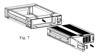
5-2. Push carrier body further into cartridge frame until fully inserted. (Fig. 8)
